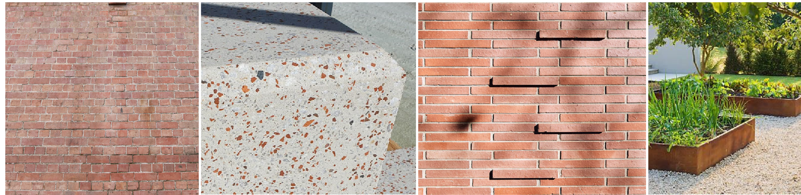
Existing Red Brick Wall Exposed Red Aggregate Concrete Proposed Red Brick Wall Corten Steel Garden Edge / Planter Wall
