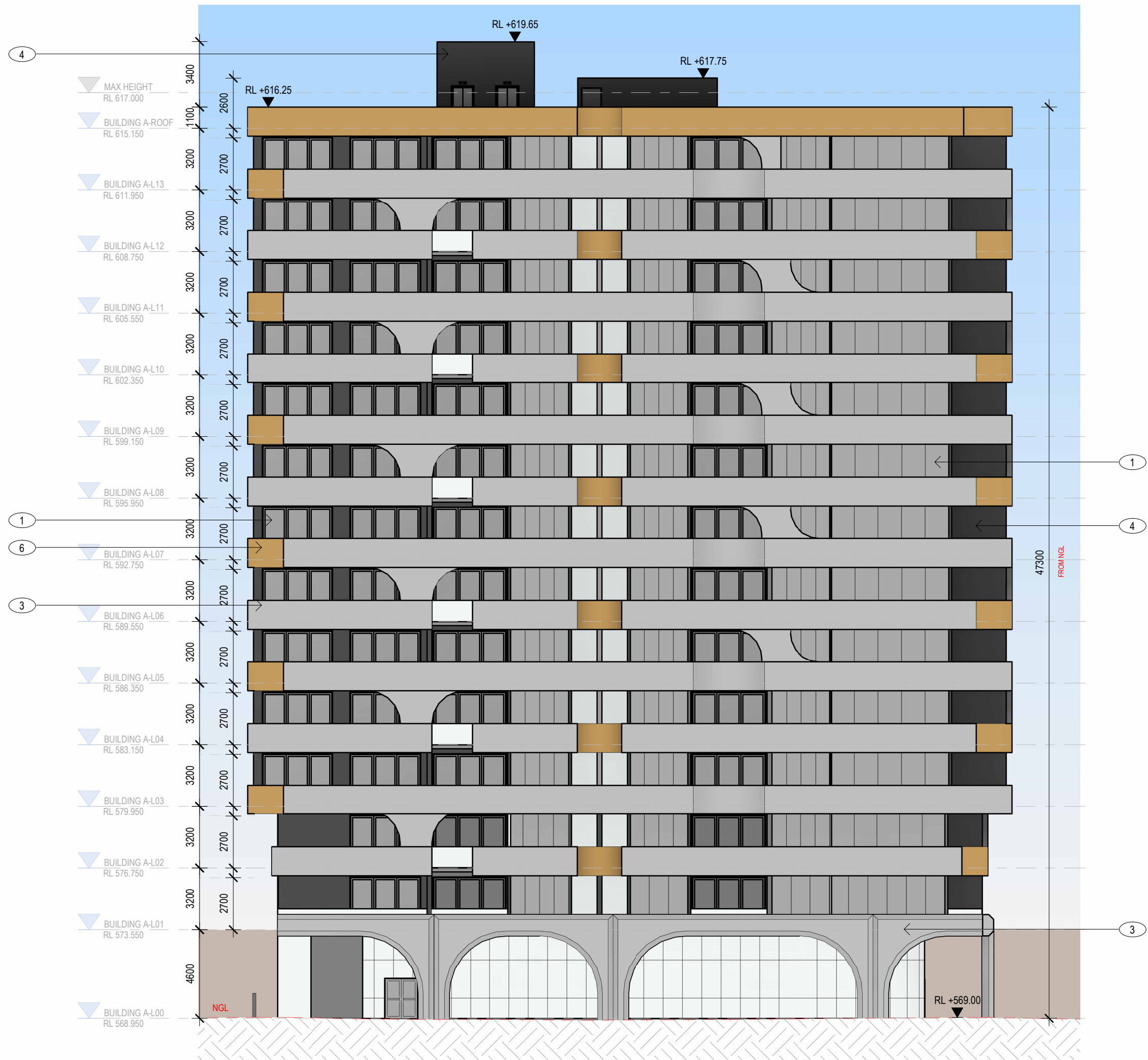
1 BUILDING A NORTH ELEVATION 1 : 200
