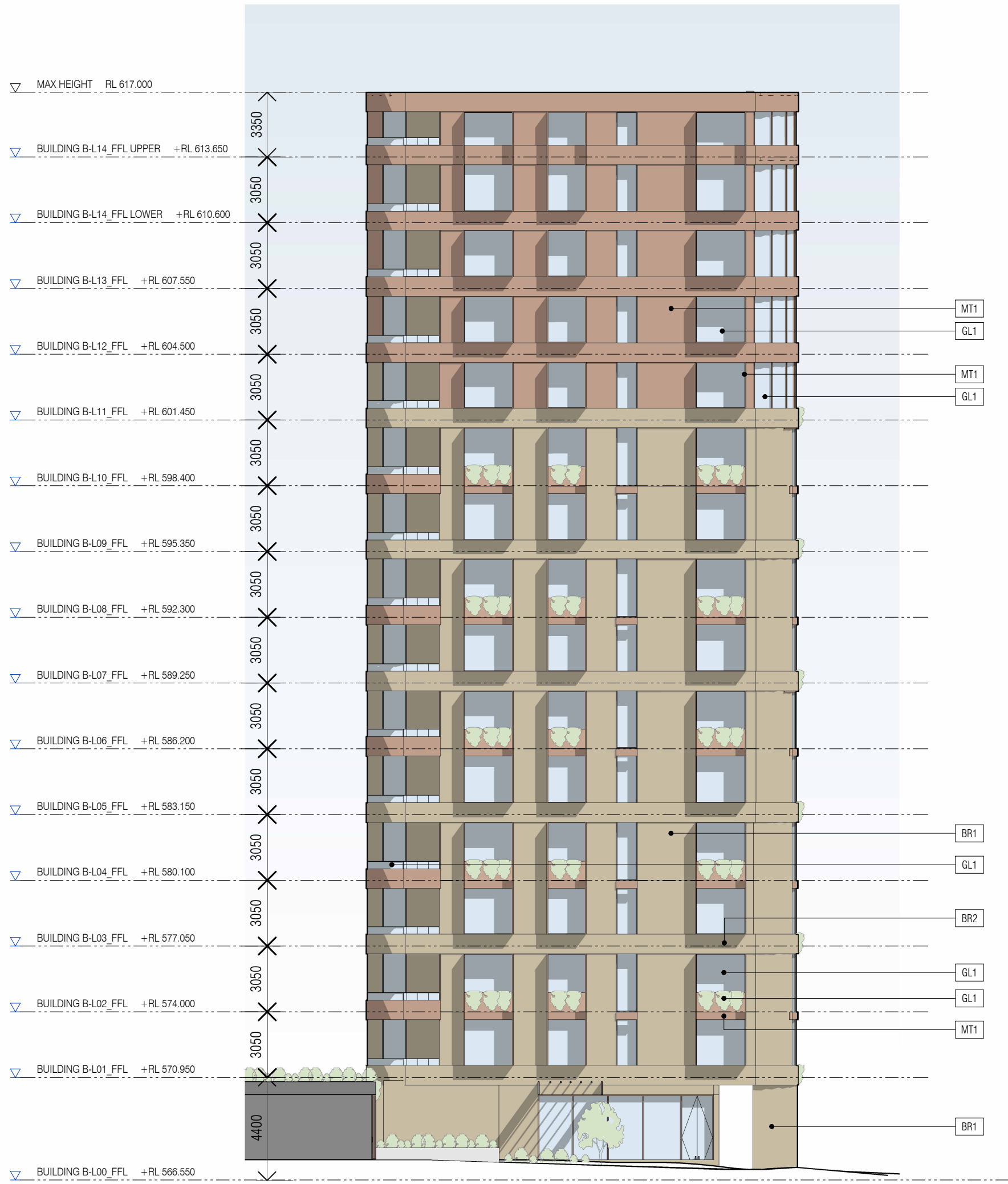
1 BUILDING B-NORTH ELEVATION DA.08.02 1 : 200 @ A1
