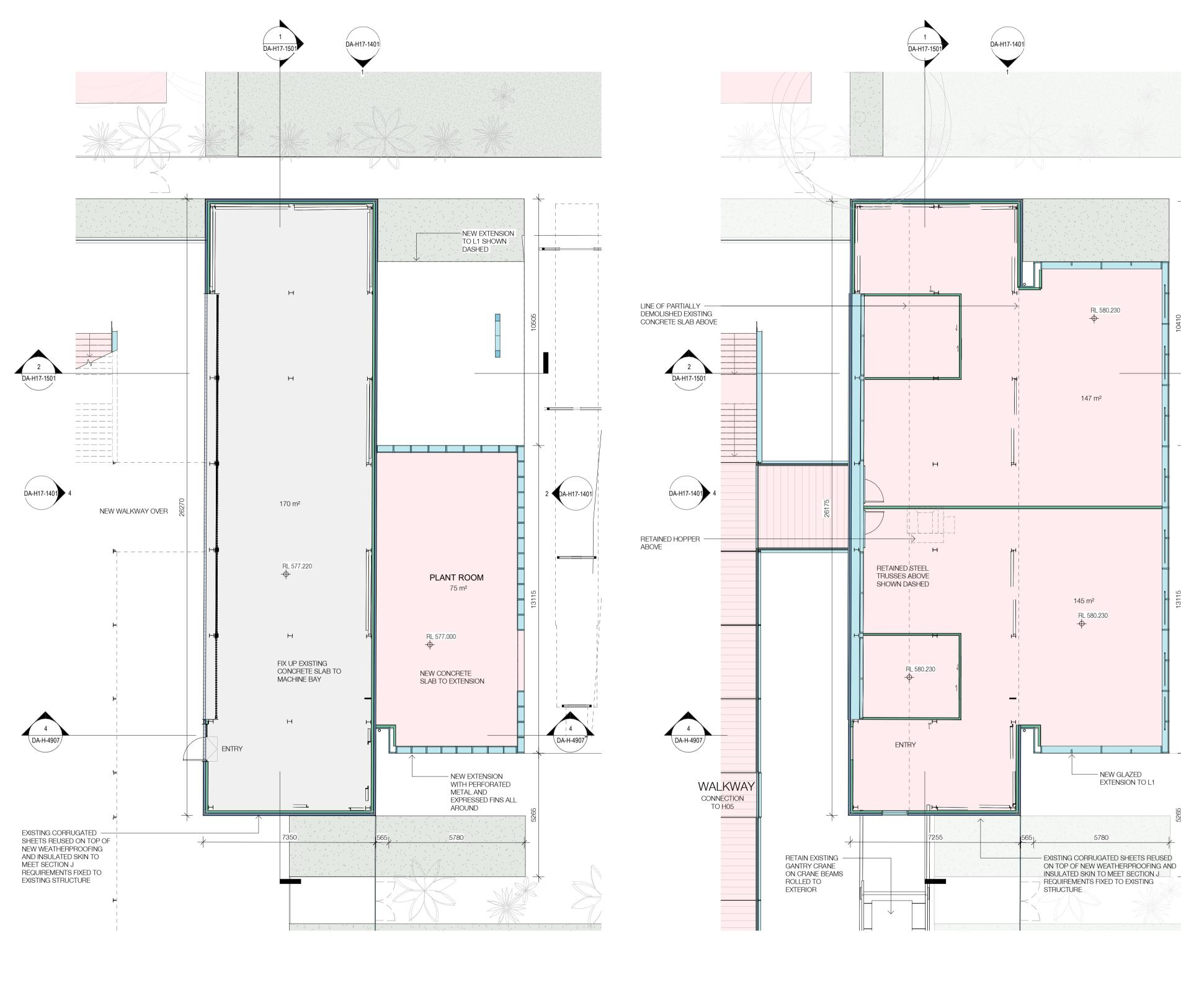
RL 590.685 RL 580.935 DA-H17-1401 4 ROOF OVER NEW WALKWAY RL 588.234 MAKE SAFE CONVEYOR BELT -STRUCTURE AND RETAIN IN PLACE ON EDGE OF NEW RESIDENTIAL POOL 5780 RL 587.270 RL 588.086 - ALL NEW GUTTERS AND DOWNPIPES TO MACHINE BAY BUILDING WILL BE CONCEALED AND HIDDEN BEHIND REUSED CORRUGATED TO MACHINE BAYS I, II and III (H15, H16 & H17): \* EXTERNAL CORRUGATED METAL CLADDING
