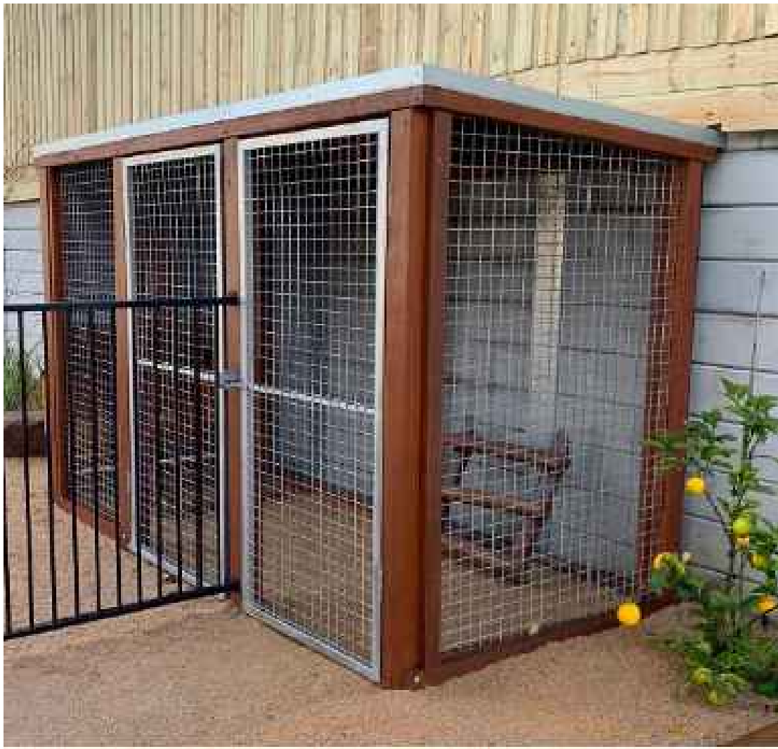
1 PROPRIETARY FURNITURE: CHICKEN COOP SCALE: NTS MANUFACTURER: Lypa MODEL: N/A SLATS: Timber FRAME: Galvanised steel SIZE: 3900mm L x 1200mm W x 1950mm H INSTALLATION: Subsurface, to manufacturer's specification
