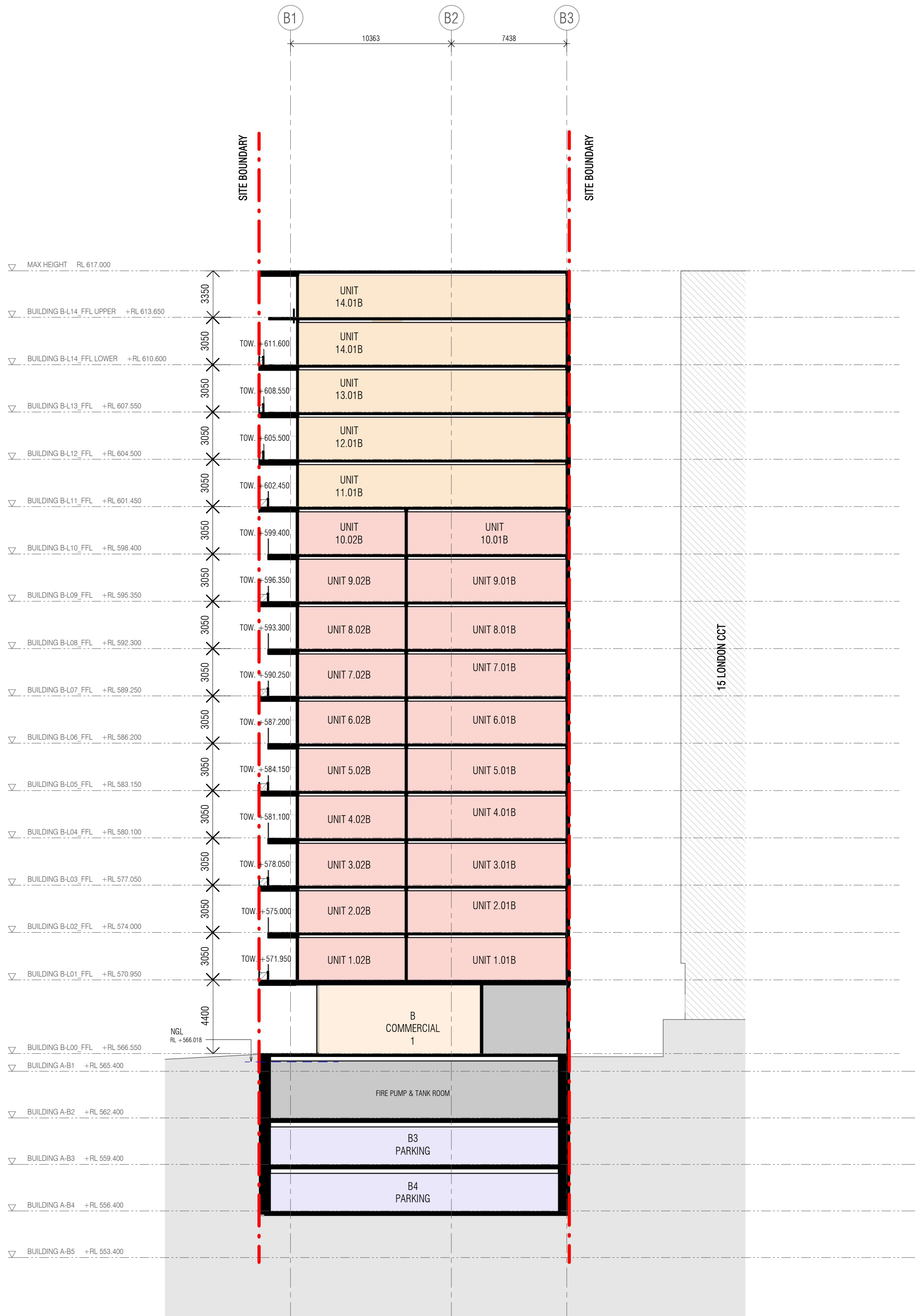
2 BUILDING B SHORT SECTION 2 DA.09.02 1 : 200 @ A1
