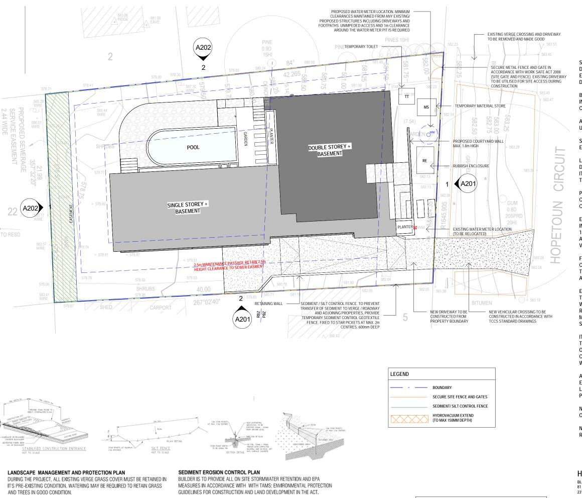
PROVIDE TEMPORARY 1.8m HIGH FENCING ON VERGE DURING CONSTRUCTION. NO CONSTRUCTION MATERIAL IS TO BE STORED ON VERGE OR PUBLIC OPEN SPACE. NO CAR PARKING OR EQUIPMENT PERMITTED ON VERGES OR ADJACENT PARKLAND.
