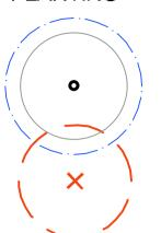
EXISTING RETANED TREE: To be retained and protected. Refer Tree Management and Protection Plan
