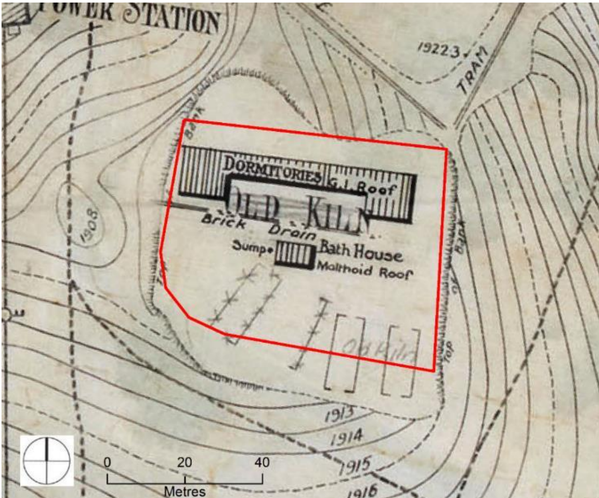
Figure 3.15 A 1916 site plan aerial showing the location of BRW8 and former structures. (Source: NAA: A6664, L165A, 1916)
