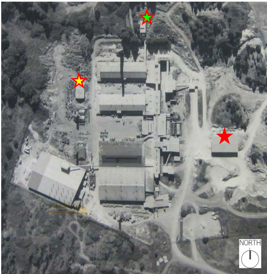
Figure 160 Aerial photograph, 1976, with the following later site elements indicated; clay storage shed (red star); coal storage bunker (red/green star) and former forklift shed (red/yellow star).
