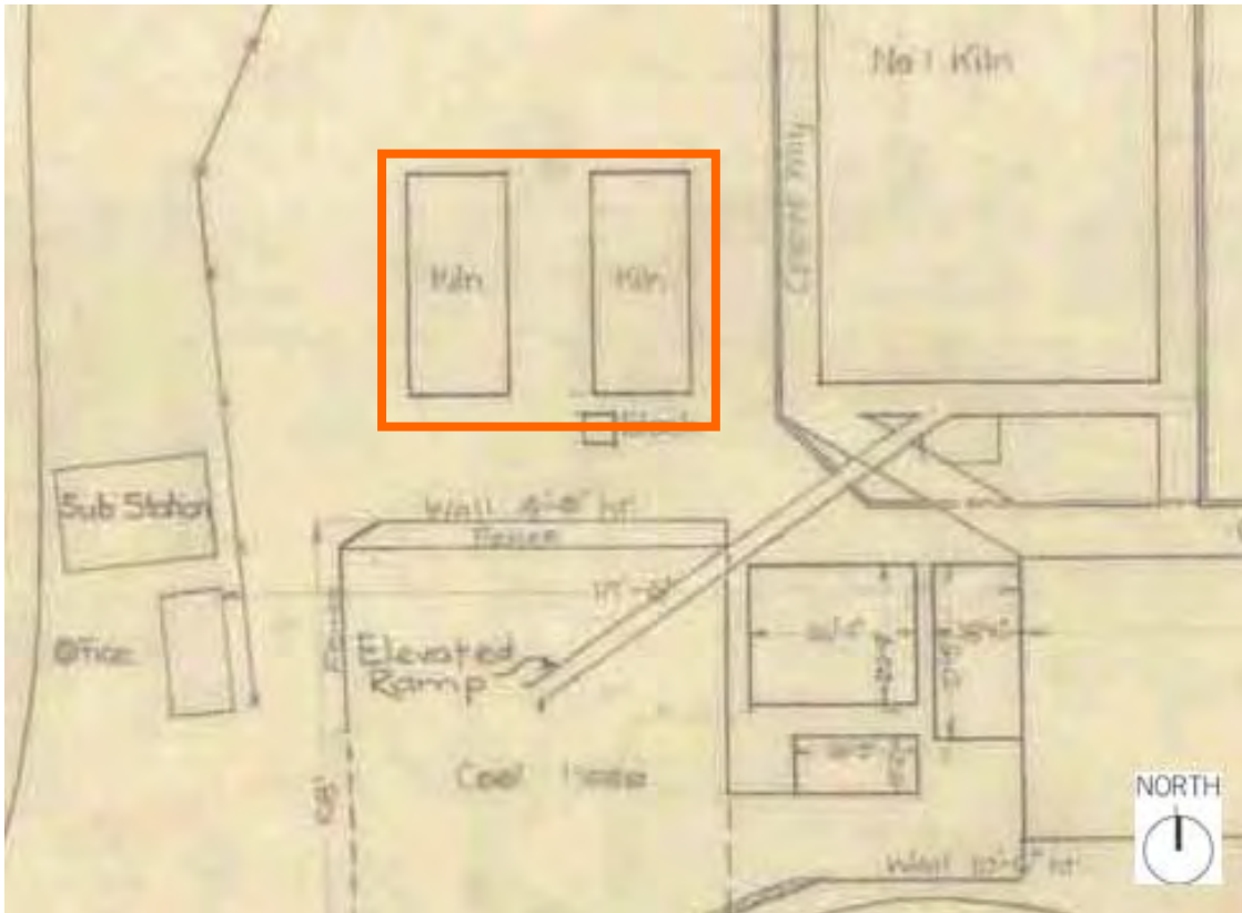
Figure 73 Detail of 1947 site plan, indicating the location of the two ‘temporary’ Downdraught kilns, to the south of the Staffordshire kiln (‘No. 1 Kiln’). . Source: National Archives of Australia.
