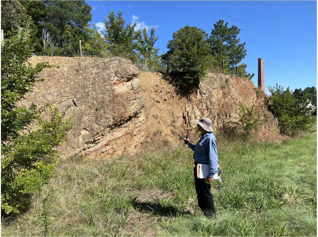
Photo 6 – 22/2/2021 – View of Locations 4A and 5A, showing the rock face to comprise foliated, HW to MW Phyllitic Mudstone, with some beds of Sandstone & Mudstone.
