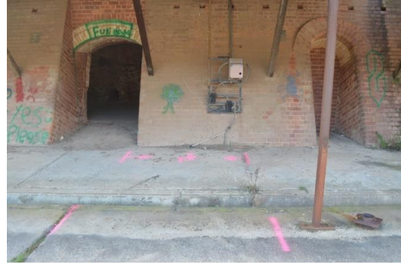
Figure 4.125 GPR identified a single tunnel leading from the fan houses to the kiln, which enters the kiln at the location of the 'Kent' oxygen analyser.
