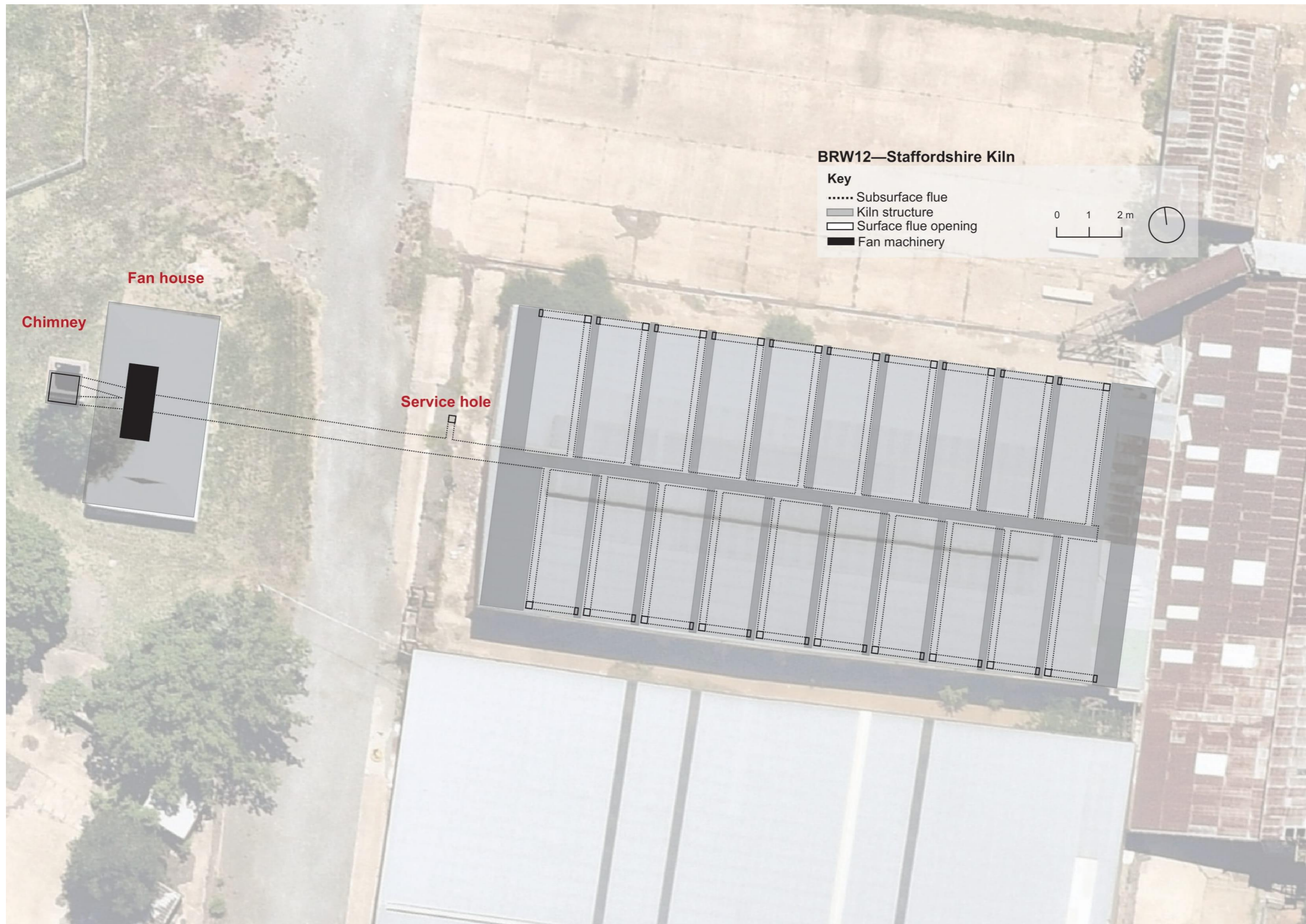
Figure 4.124 The subsurface flues for the Staffordshire Kiln.
