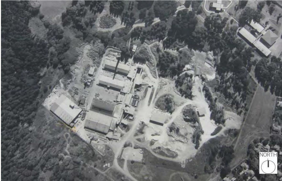
Figure 2.12 An aerial photograph of the Brickworks in 1976, the year of its closure. The photograph shows the six extant kilns, the extrusion plant to the west, a number of sheds within the quarry, and a carpark at the entrance of the complex. (Source: ACT Heritage Library)
