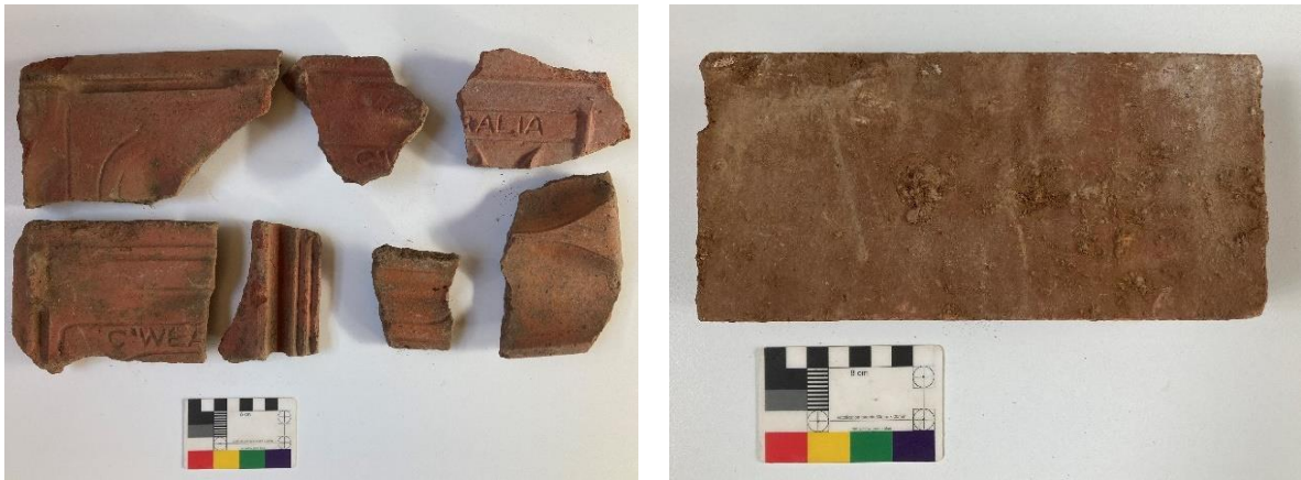
Figure 4.144 Other building materials made at the Precinct include 'C'WEALTH' roof tiles (far left), 'AUSTRALIA' roof tiles (centre left), and common pavers (right).
