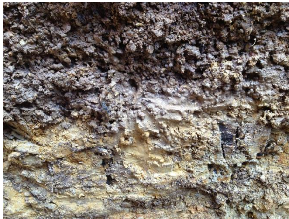
Photograph 6: Saturated gravelly clay, TP3
