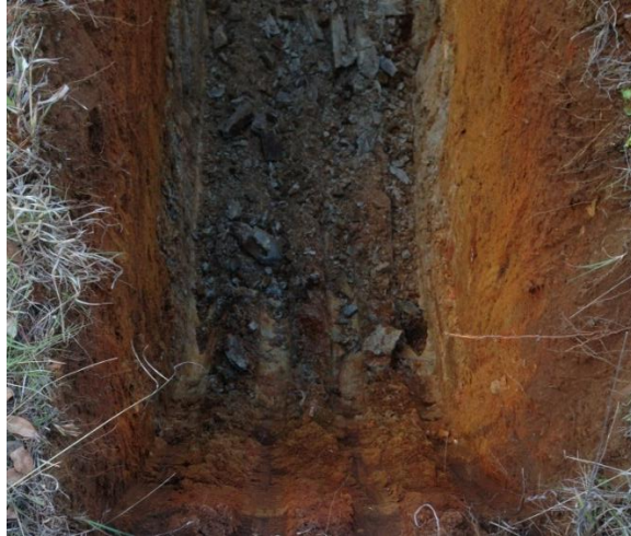
Photograph 5: Orange brown and red brown clays typical of the residual soil overlying siltstone. TP18.
