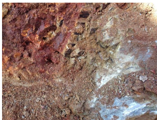
Photograph 8: Corestone of fresh high strength siltstone (bottom right) surrounded by highly weathered, low strength siltstone. TP17
