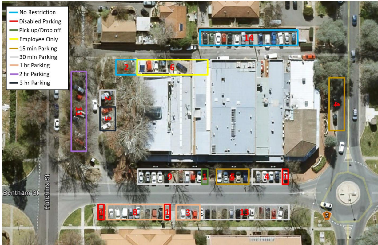
Figure 7 Yarralumla shops parking restrictions and Supply (2021)
