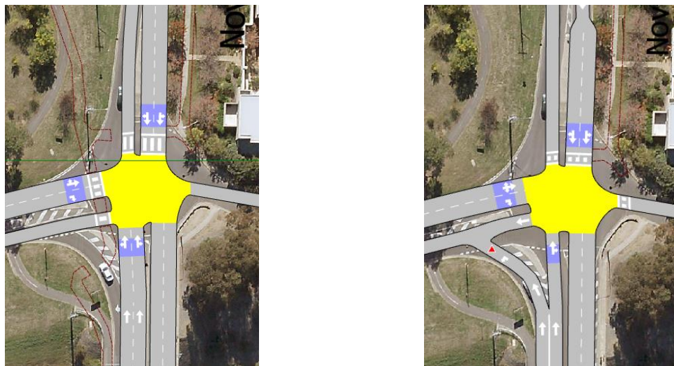
Figure 18: Change in layout to test the effectiveness of providing a signalised left turn lane from Kent Street to Dudley Street
