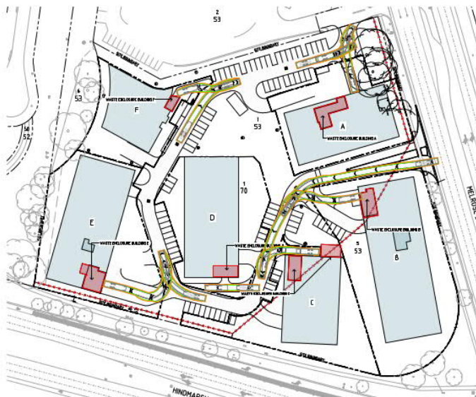
Figure 6.3 Swept paths - service access arrangement (waste collection)
