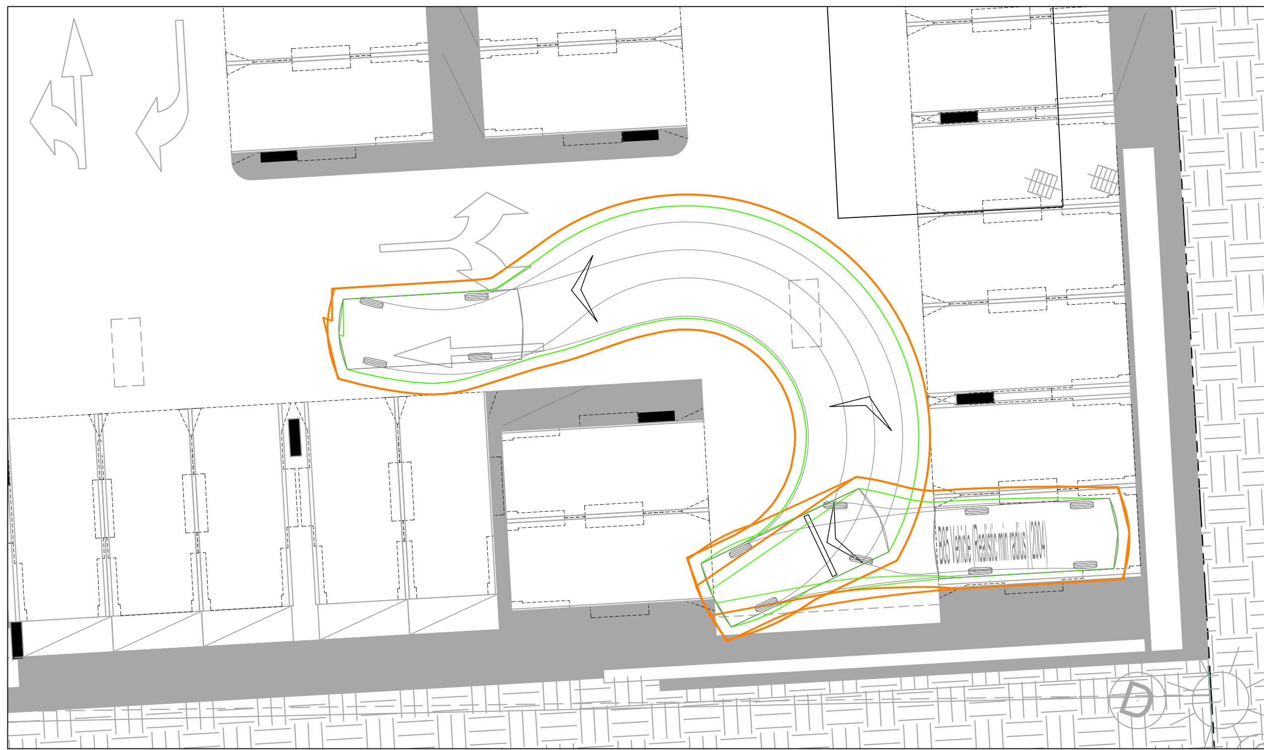
B85 EXIT FROM PARKING BAY SCALE 1:200
