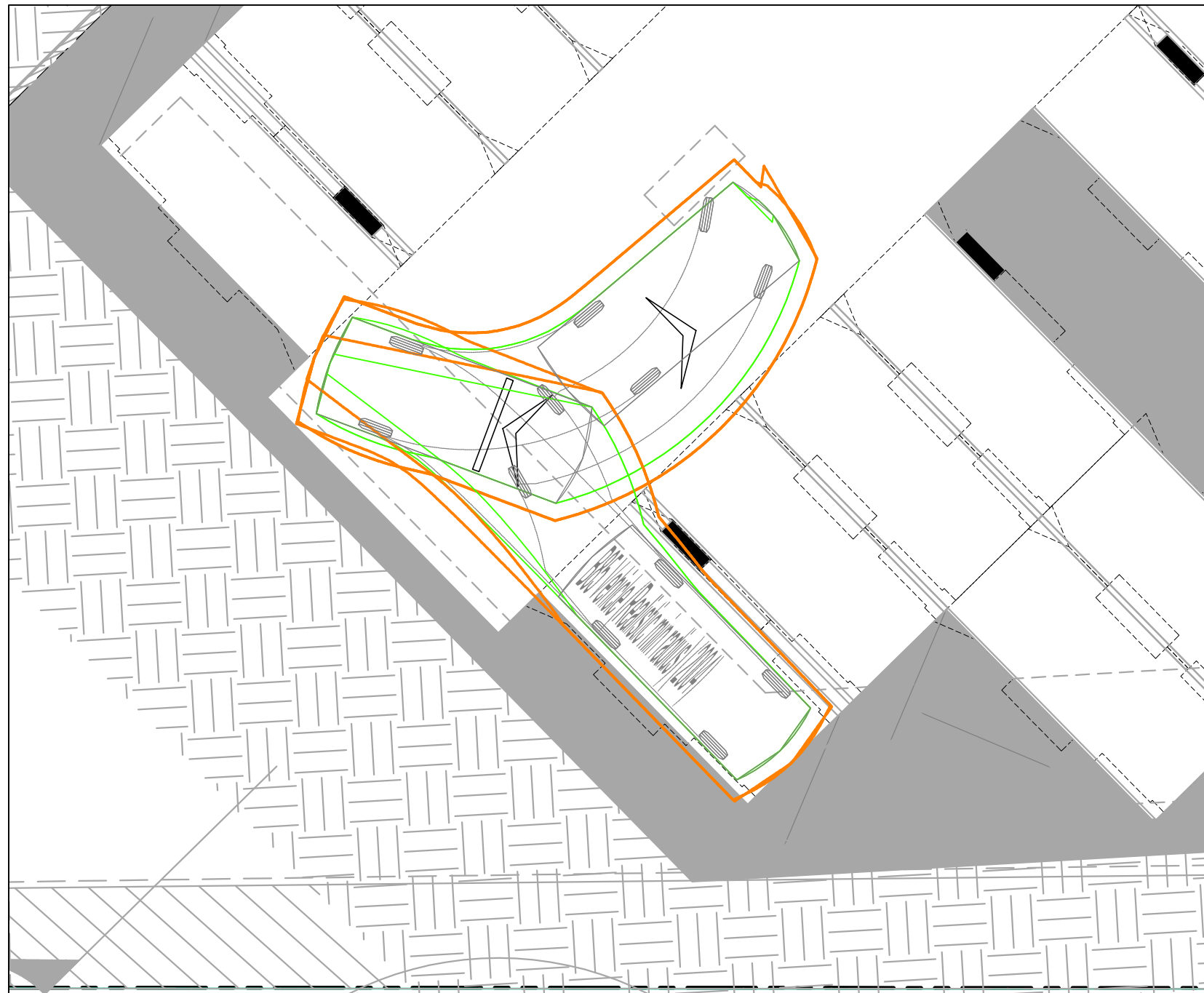
B85 EXIT FROM PARKING BAY SCALE 1:200
