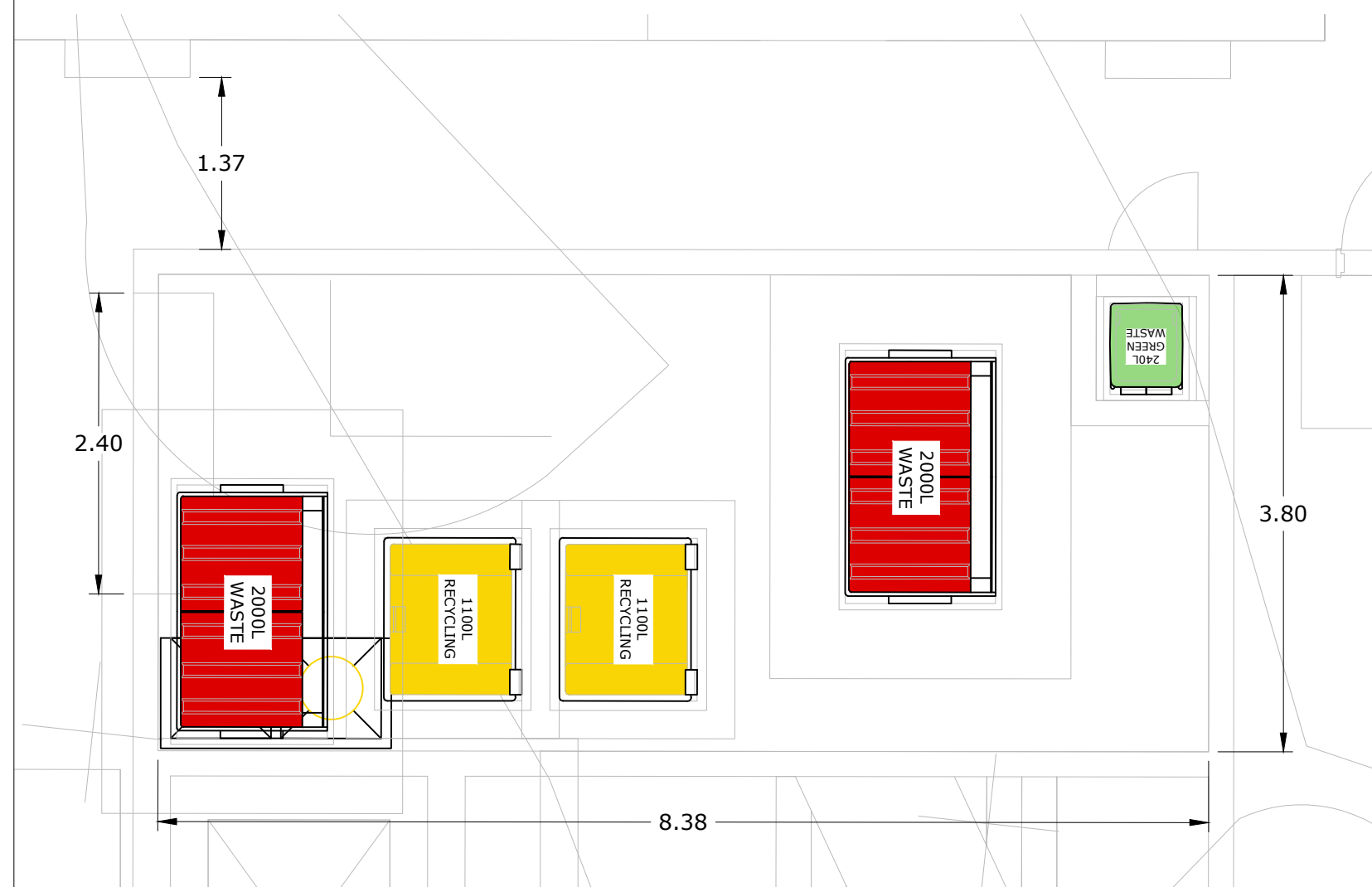
BUILDING 'D' SATELLITE ENCLOSURE PLAN (CHUTE)
