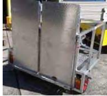
Conditional registration kit including Tail & Brake lights, Indicators, Reflectors & Number plate light.
