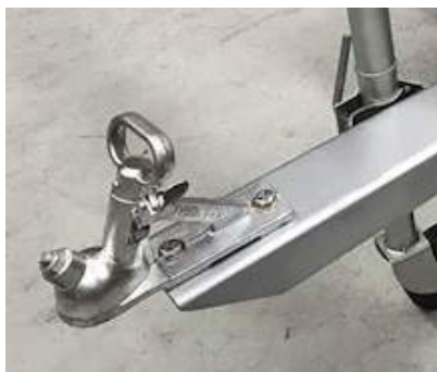
Adjustable height heavy duty draw-bar pre-drilled to suit standard connection types: 50 mm towbar hitch Or Drop-in pin hitch.
