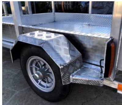
8 Inch Alloy Wheels with Holden precision bearings & Highway grade 6 ply tires designed to resist side loads on ramp. Complete with Wheel Guards for protection and road safety.
