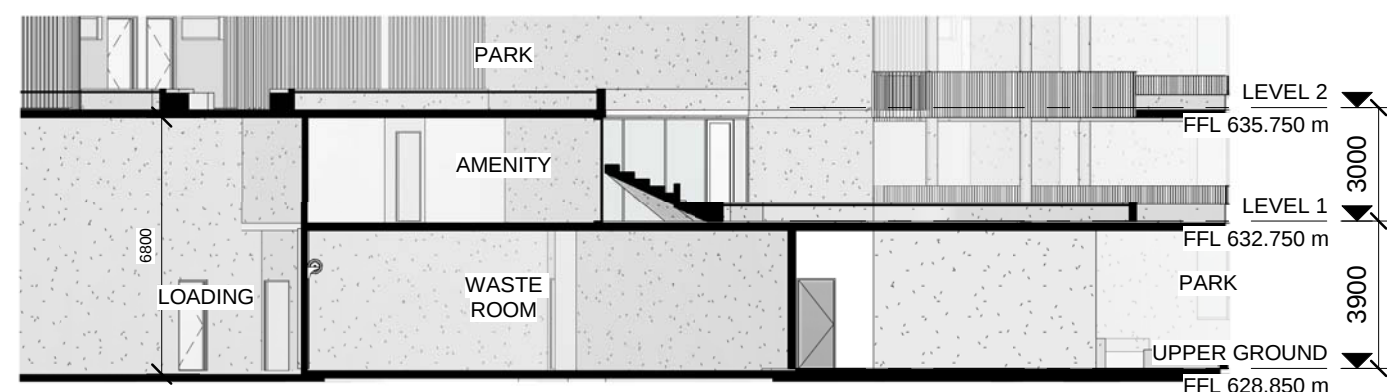
4 SECTION H - WASTE ENCLOSURE SCALE 1 : 200
