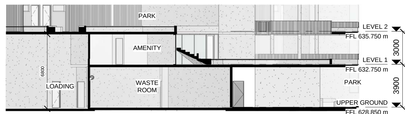
4 SECTION H - WASTE ENCLOSURE SCALE 1 : 200
