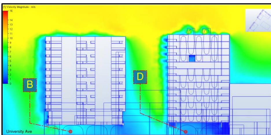
Figure 4.7 CFD modelling results for Scenario 2: westerly at 40km/h at section view
