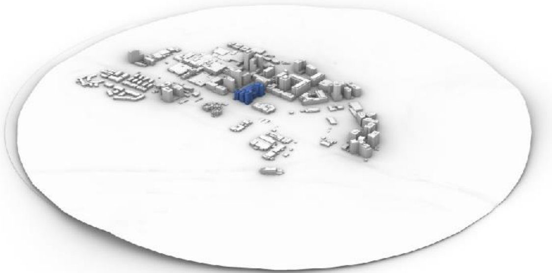
Figure 3: CFD Domain modelled for the Woden Village development. The development is shown in blue.
